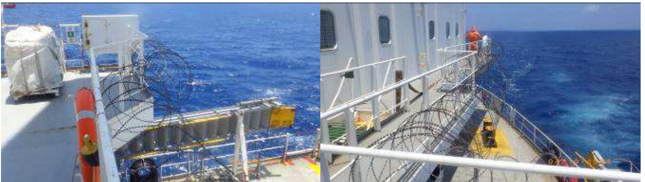
RAZOR WIRES RIGGED AROUND "A DECK" FOR ADDITIONAL PROTECTION
